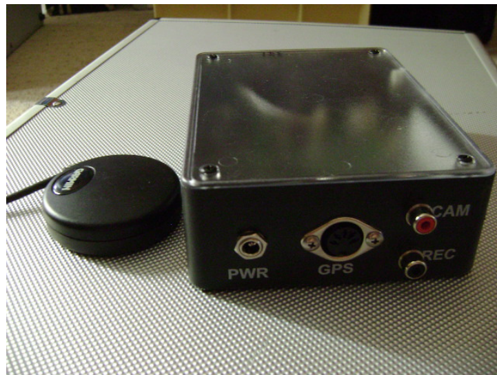
Garmin-18 GPS unit, and KIWI system
