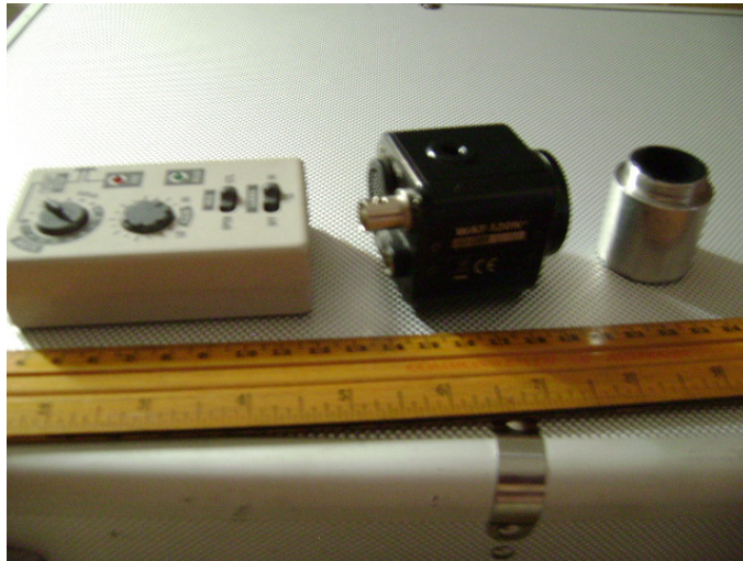
Waterc 120N+ control box, camera body, and 1 1/4" adaptor
