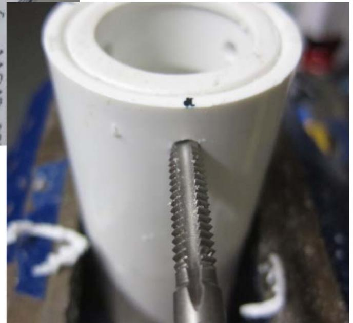
Plastic is soft, you can drive the tap in and out with a reversing drill.
