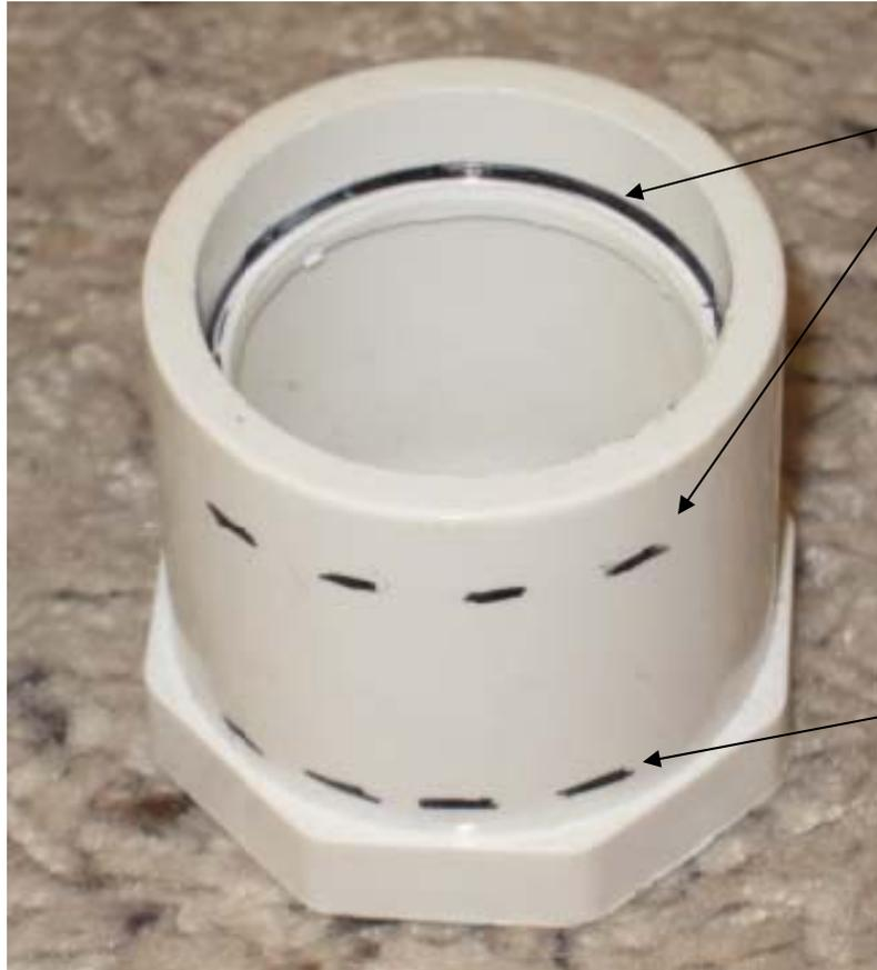
Cut through adapter even with black line to leave inner ring flush with the new cut end. This inner ring will serve as a stop for the 1 ¼" camera focal reducer.
