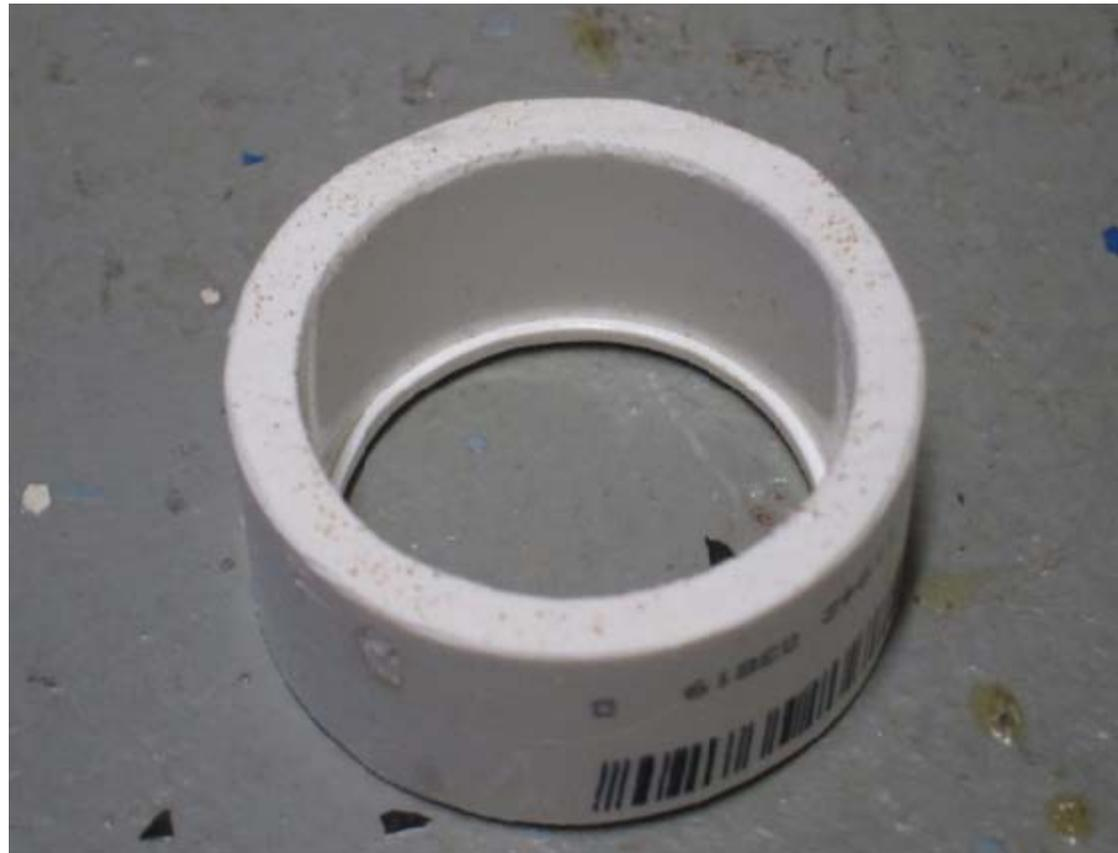
Place a small ring of cement on the inside of one end of the glued-up coupling (doesn't matter which end)
