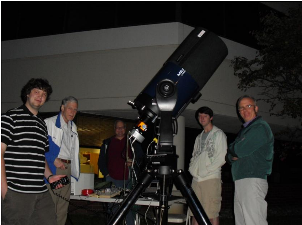
After dinner, we set up two scopes and attempted to record some lunar occultations. Conditions were clear, but the 92% disk and slight lunar haze washed out the targets. Above, a 12" LX200 with an Andor Luca-S emCCD camera is shown. (l-r) Dylan, David, Don, Kevin Gruber, and Steve.
