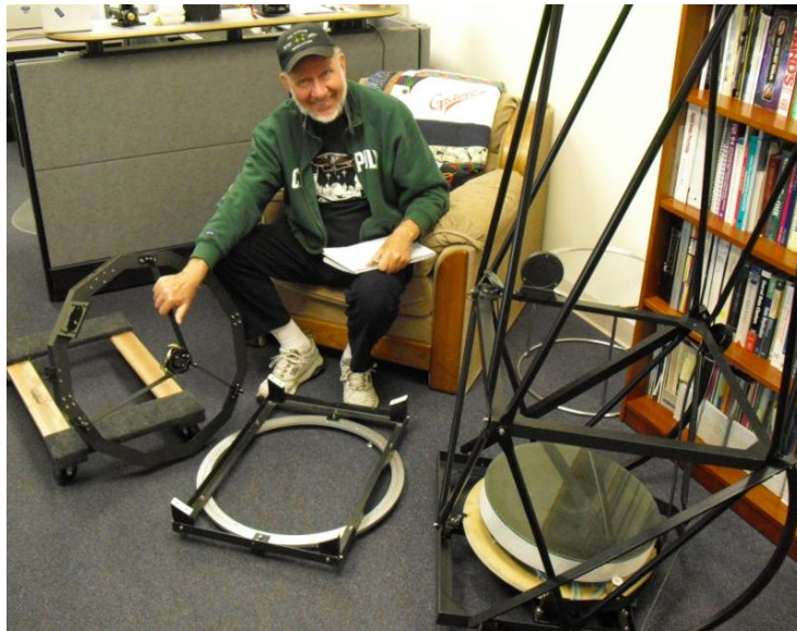
The UL20 is disassembled into major pieces. The OTF Designs foamglass mirror is setting on a “pneumatic warping harness” prototype. Russ is holding the top end and made suggestions for motorizing the axes.
