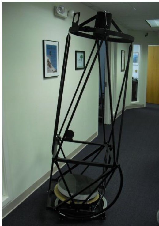
Hubble Optics UL20 lightweight mount with an 18" OTF Designs foamglass mirror (uncoated) on a pneumatic warping harness. The whole telescope (and mount) weighs under 75 lbs and is very portable.
