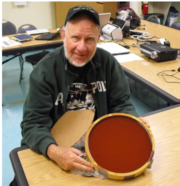
Russ holds an 11” spun epoxy mirror just fabricated by Lisa Brodhacker at Lander U. Gravic will conduct the mirror quality tests.
